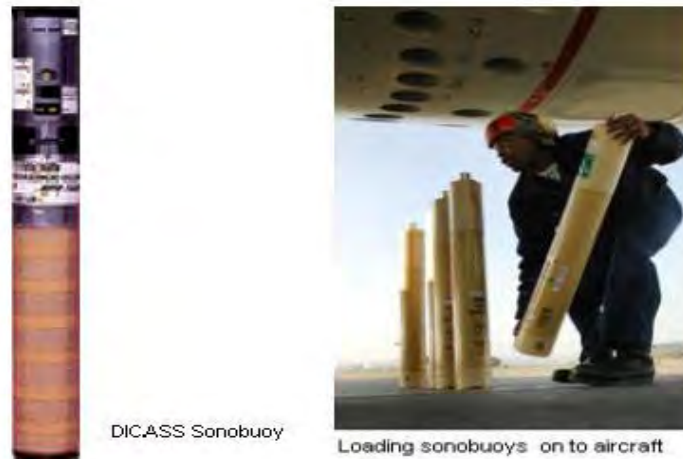
Figure 2.3-3: Sonobuoys (e.g., AN/SSQ-62)
