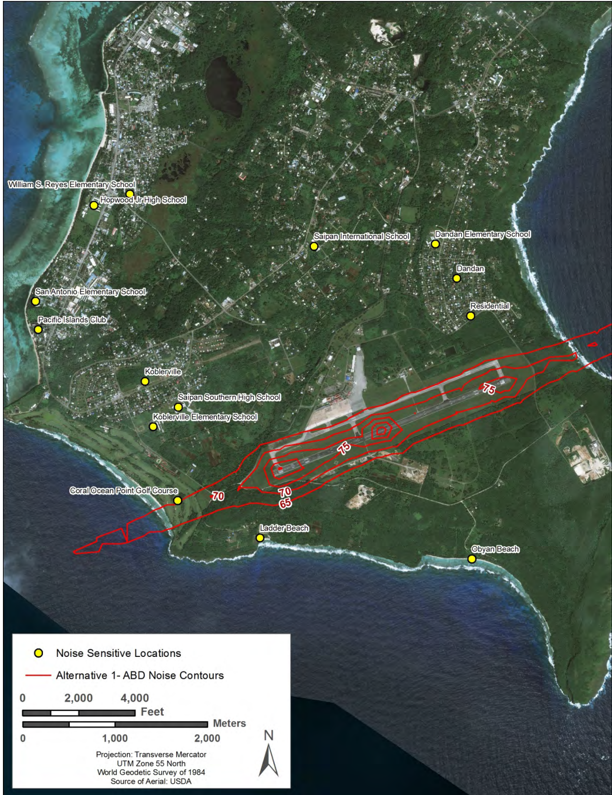
Figure 4.10-4. Noise Sensitive Locations near Saipan International Airport with Alternative 1-ABD Noise Contours
