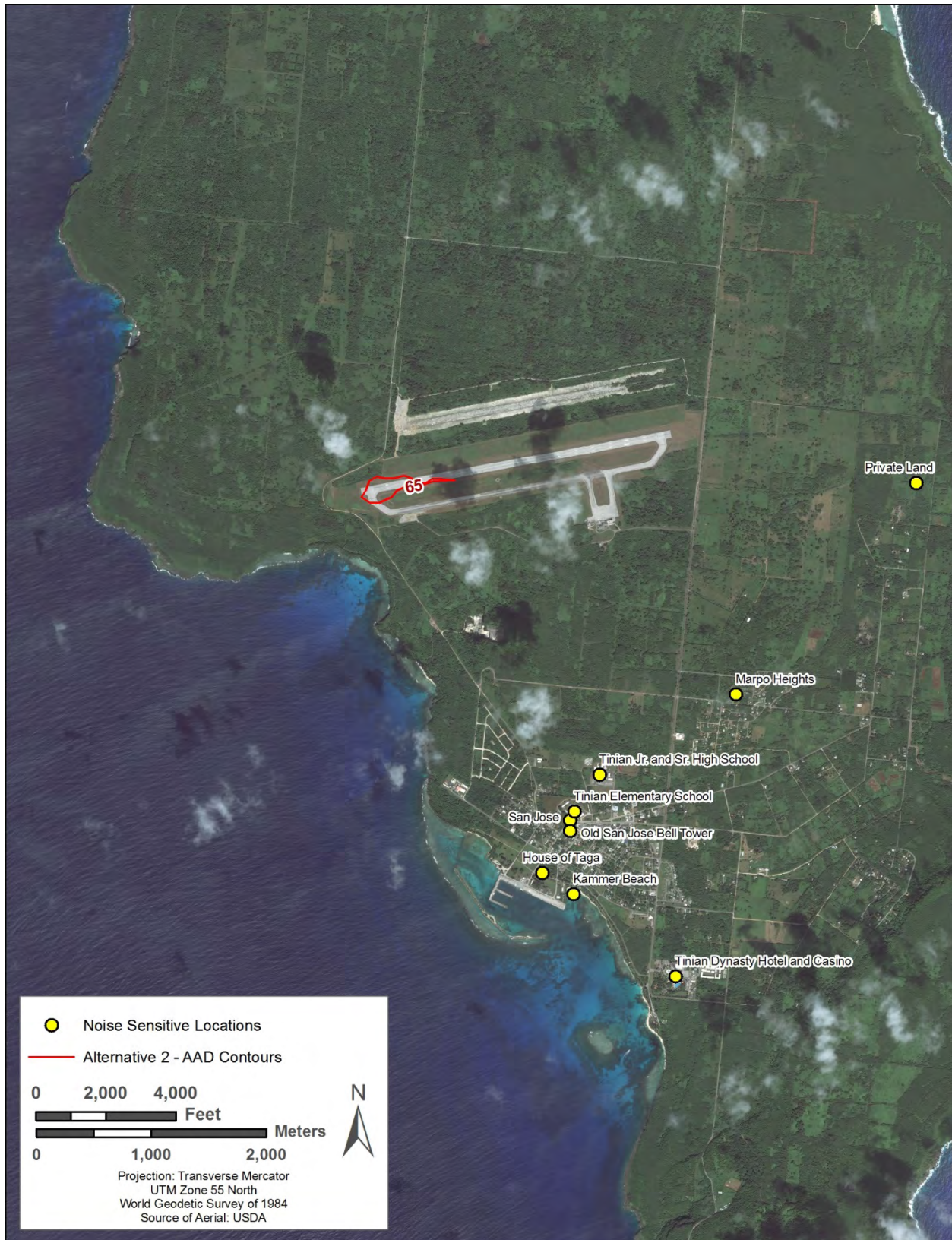
Figure 4.10-6. Noise Sensitive Locations near Tinian International Airport with Alternative 2-AAD Noise Contours
