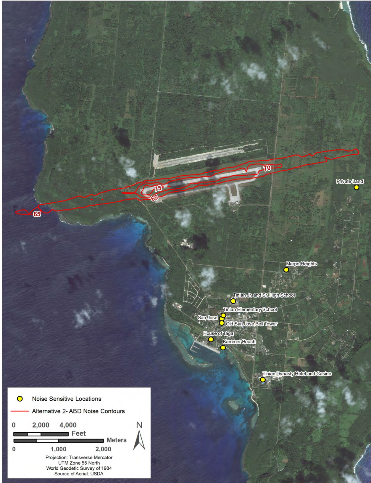
Figure 4.10-8. Noise Sensitive Locations near Tinian International Airport with Alternative 2-ABD Noise Contours
