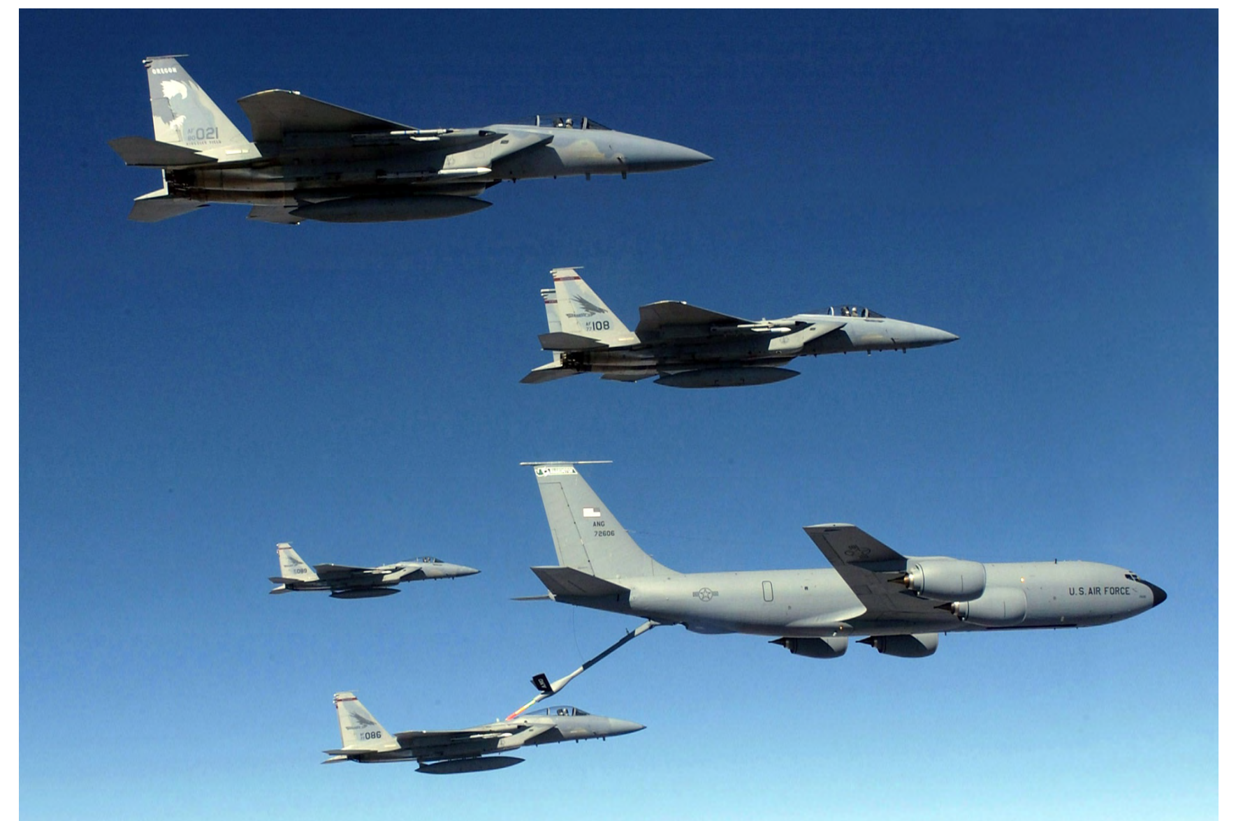
A KC-135 Stratotanker aircrew refuels four F-15 Eagles over Afghanistan. In 2008, Air Force tankers passed more than 1 billion gallons of fuel to coalition aircraft. (U.S. Air Force photo/Staff Sgt. James L. Harper Jr.)
